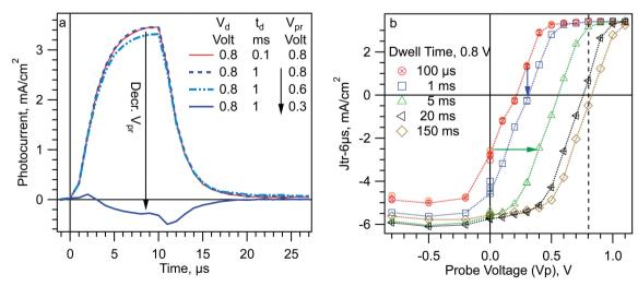
Fig. 4 Results of SDSP experiments on a planar MAPI cell. (a) Example photocurrent transients for a dwell voltage ( $V_d$ ) of 0.8 V. (b)  $J_{tr}$ -6 $\mu$ s vs.  $V_{pr}$  and  $t_d$ . from SDSP experiments using a dwell voltage of 0.8 V.
