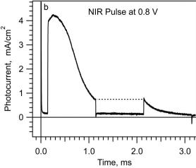
Photocurrent transients from longer light pulses. Transients from the same planar cell shown in Fig. 1 and 2. Pulses from a 735 nm LED
