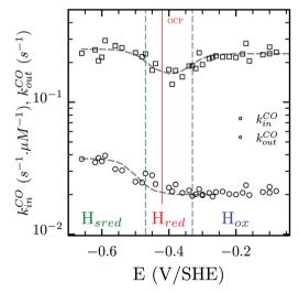
Fig. 5 Redox dependence of rate constants  $k_{in}$  and  $k_{out}$  from Scheme 1. The vertical lines mark the positions of the reduction potential of H<sup>+</sup>/H<sub>2</sub> couple at pH 7 (red) and the redox transitions undergoing at the H-cluster according to ref. 31 (we assume  $\Delta E_{\mathrm{Hox/H_{red}}}^0 = -60 \mathrm{\ mV}$  per pH unit).
