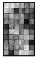
Fig. 13 EL images of c-Si PV modules after a chamber PID test under high humidity and temperature conditions (A) and after a PID test with an Al foil (B). The dark squares are the cells which are shunted due to PID. Prior to PID testing, both modules were in good condition with no shunted cells.
