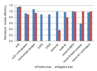
Fig. 18 Normalised PV module efficiencies after the positive or negative voltage-biased damp heat tests. The normalisation is relative to the module's measured efficiency before the PID test. 10 different types of commercial modules are tested with both positive and negative biasing. The CdTe and CIGS modules exhibited 0% efficiency after negative bias. Reprint from ref. 40. Copyright 2011, Elsevier.
