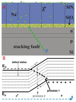
Fig. 6 (A) Schematic drawing of a solar cell cross section and transport of  $\mathrm{Na}^+$  (green dots) through the  $\mathrm{SiN}_{x}$  layer and subsequent diffusion into the stacking faults. (B) The proposed band structure along a Na decorated stacking fault. Reprint from ref. 65. Copyright 2014, Elsevier.
