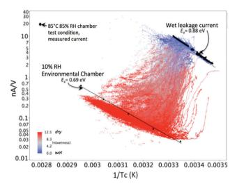
Fig. 20 System voltage-normalized current over a period of about six months for a module held by edge clips (frameless) in Florida, USA (redblue data, where blue is wet and red is dry according to the wetness sensor). Results in a dry chamber (10% RH, five lower points), wet leakage current tests (upper data), and for the 85 °C/85% RH chamber test conditions performed on a sister module are superimposed in black. Reprint from ref. 126. Copyright 2016, IEEE.
