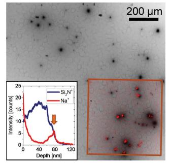
Fig. 4 An EBIC image of a monocrystalline silicon cell region with a high density of PID shunts acquired at an acceleration voltage of 30 kV. The inset shows the distribution of Na at the SiN<sub>x</sub>/Si interface measured by the ToF-SIMS. Reprint from ref. 65. Copyright 2014, Elsevier.
