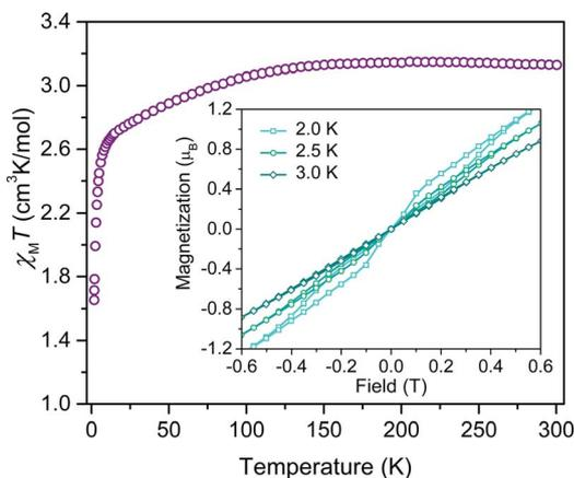
Fig. 2 Temperature dependent magnetic susceptibility ( $\chi_M T$ ) of a polycrystalline powder of **4** collected under an applied field of 0.1 T. Inset: overlay of hysteresis curves collected on **4** at 2 K, 2.5 K, and 3 K at a scan rate of 8 mT s<sup>-1</sup>.
