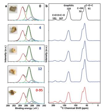
Fig. 1 (a) C 1s XPS spectra and photographs (inset), and (b) magicangle spinning <sup>13</sup>C ssNMR spectra of different freeze-dried GO-n and GO-0-95 samples; the values of n are depicted in (a).
