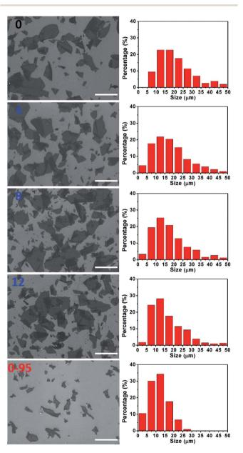
Fig. 3 Typical SEM images and corresponding histograms of GO size distributions (right to the SEM image) of GO-n and GO-0-95 samples; the values of n are depicted in the panels; scale bar, 50  $\mu$ m. The histograms of GO size distributions were obtained by counting more than 200 sheets for each sample.
