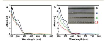
Fig. 7 UV-Vis spectra of (a) fresh  $H_2SO_4$  solutions of KMnO $_4$  containing 0 (black), 4 (blue), 8 (green), and 12 mL (red) water at 0 °C, respectively, and (b) after keeping them at 40 °C for 2 h. Inset in (b) shows the photographs of the corresponding solutions in capillary tubes.
