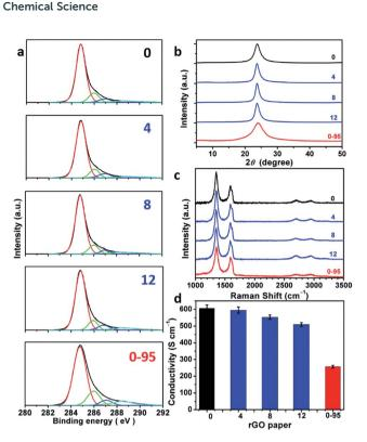
Fig. 5 (a) C 1s XPS spectra, (b) XRD patterns, (c) 514.5 nm excited Raman spectra, (d) conductivities of rGO-n and rGO-0-95 papers; the values of n are depicted in the figure.
