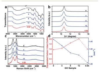
Fig. 2 (a) ATR-FTIR spectra, (b) XRD patterns, (c) 514.5 nm excited Raman spectra, (d) atomic ratio of oxygenated carbons/intact carbons and mean distance between two defects ( $L_D$ ) of GO-n and GO-0-95; the values of n are depicted in the figure.
