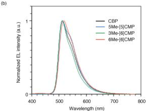
Fig. 5 Performance of the single-layer OLED. (a) External quantum efficiency of the single-layer OLED plotted against the current density. See Fig. 1a for the device architecture. (b) Electroluminescence spectra at a current density of  $0.1 \, \text{mA cm}^{-2}$ .
