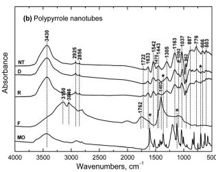
Fig. 5 Infrared spectra of (a) globular (G) and (b) nanotubular polypyrrole (NT) before and after deprotonation with 1 M ammonium hydroxide (D), and reprotonation with 1 M hydrochloric acid (R). Spectra of the solids collected from filtrate after deprotonation (F) and of neat methyl orange (MO) are included for comparison.
