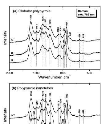
Fig. 7 Raman spectra of (a) globular (G) and (b) nanotubular (NT) polypyrrole before and after deprotonation with 1 M ammonium hydroxide (D), and reprotonation with 1 M hydrochloric acid (R).
