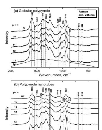
Fig. 10 Raman spectra of original (a) globular (G) and (b) nanotubular polypyrrole (NT) and after exposure to the medium of various pH.
