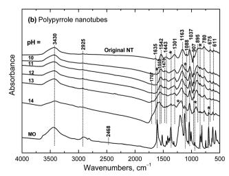
Fig. 9 Infrared spectra of (a) globular and (b) nanotubular polypyrrole before and after exposure to the media of various pH.
