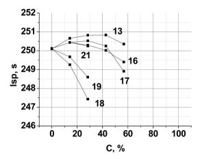
Fig. 6 Calculated specific impulse of (AP + new compound)-Al(20%)-HCB(9.5%) propellants over various new compound loadings. Here, C is the percentage of a new compound in the mixture with AP. HCB is hydrocarbon binder ( $C_{73.17}H_{120.9}$ ,  $\Delta H_f^{\circ} = -393 \text{ kJ kg}^{-1}$ ,  $\rho = 0.91$  $g cm^{-3}$ ).44
