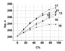
Fig. 7 Calculated specific impulse  $I_{\rm sp}$  of (AP + new compound)-Al(20%)-AB(14-15%) propellants over various new compound loadings. Here, C is the percentage of a new compound in the mixture with
