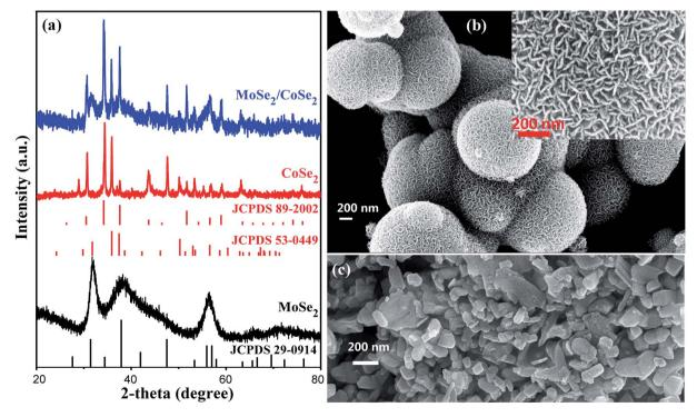
Fig. 1 (a) XRD patterns of the as-synthesized pure MoSe<sub>2</sub>, CoSe<sub>2</sub>, and MoSe<sub>2</sub>/CoSe<sub>2</sub> composite; (b) and (c) are SEM images of the as-synthesized pure MoSe<sub>2</sub> and CoSe<sub>2</sub>, respectively.
