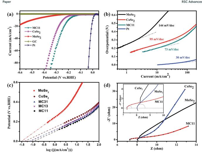
Fig. 3 (a) Polarization curves and (b) corresponding Tafel plots of MoSe<sub>2</sub>, CoSe<sub>2</sub>, and MC11, respectively. The polarization and Tafel data derived from blank GC electrode and Pt were given for comparison. (c) Calculated exchange current densities of various samples by applying extrapolation method to the Tafel plots. (d) Nyquist plots of various samples. The partial circle data was fitted with the simplified Randles equivalent circuit<sup>6</sup> using EC-lab software.
