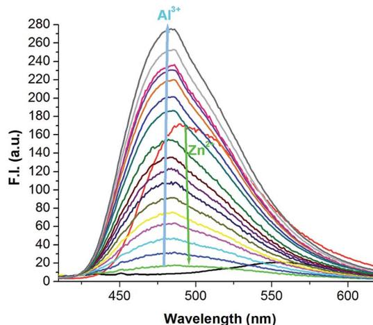
Fig. 5 Selectivity for  $\text{Al}^{3+}$  over the  $\text{H}_2\text{SAL-NH-Zn}^{2+}$  complex.
