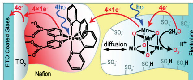
Fig. 22 Schematic depiction of the photoelectrochemical cell containing Mn cubane 40 . Reprinted with permission from ref. 160. Copyright 2010 American Chemical Society.
