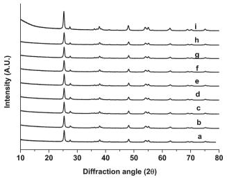
Fig. 2 XRD patterns of (a) TiO<sub>2</sub> P25 (b) 5% Ru/TiO<sub>2</sub> (c) 4% Ru-1% Pd/ TiO<sub>2</sub>, (d) 3% Ru-2% Pd/TiO<sub>2</sub>, (e) 2.5% Ru-2.5% Pd/TiO<sub>2</sub>, (f) 2% Ru-3% Pd/TiO2, (g) 1% Ru-4% Pd/TiO2, (h) 0.5% Ru-4.5% Pd/TiO2, (i) 5% Pd/ TiO<sub>2</sub>.
