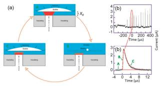
Fig. 11 (a) Sketch of bubble evolution near a surface. (b) Single bubble cavitation chronoamperometric current recorded for [Ru(NH<sub>3</sub>)<sub>6</sub>]Cl<sub>3</sub> (10 mM) in aqueous KNO<sub>3</sub> (0.1 M) under sonication at 20 kHz. Conditions: horn-to-electrode distance 7 mm, insonation power 8.9 W cm<sup>-2</sup> electrode diameter 32 µm. (c) Zoom on a single spike (circles) and simulation (line). For simplicity reduction currents are here positive. Adapted from ref. 68.
