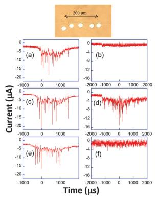
Fig. 10 Top: Example of microelectrode array. Bottom: Chronoamperometric current recorded simultaneously (a, c and e or b, d and f) on three electrodes using 50 mM K<sub>3</sub>[Fe(CN)<sub>6</sub>] in aqueous KNO<sub>3</sub> (0.1 M). Adapted from ref. 67.
