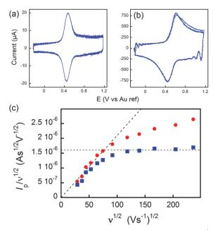
Fig. 7 (a and b) Voltammograms of  $C_{60}Fc$  at 836 (a) and 55 850 V s<sup>-1</sup> (b) in acetonitrile +1 M tetra-n-butylammonium tetrafluoroborate. (c) Peak current evolution with the scan rate. Red dots: experimental data. Blue dots: corrected data featuring a diffusion plateau at large scan rates. Adapted from ref. 62
