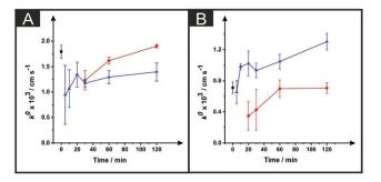
Fig. 3 The effect of drying variables (temperature and time) upon the utilising DMF-modified and unmodified (squares) ESPEs (A) and MSPEs (B). Note: prior to the DMF immersion step, the SPEs insulating layer was further protected with a DMF inert film. Experimental parameters: 20 minutes DMF modification followed by curing temperatures of: 60 °C (circles) and 100 °C (triangles). Data for the  $k^0$  were deduced using eqn (3). Represented data indicate the average and standard deviation (N = 3).
