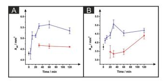
Fig. 4 The effect of drying variables (temperature and time) upon the Aeff utilising DMF-modified and unmodified (squares) ESPEs (A) and MSPEs (B). Note: prior to the DMF immersion step, the SPEs insulating layer was further protected with a DMF inert film. Experimental parameters: 20 minutes DMF modification followed by curing temperatures of: 60 °C (circles) and 100 °C (triangles). Data for the Aeff were deduced using eqn (4). Represented data indicate the average and standard devi-
