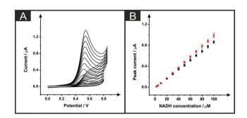
Fig. 5 Typical cyclic voltammograms (A) as a result of increasing concentrations of NADH (2.5–100  $\mu\text{M})/\text{pH}$  7.1 PBS using a DMF-modified ESPE (10 minutes within the solvent and a curing temperature of 100 °C for 30 minutes) and corresponding calibration plots (B) over the concentration range using an unmodified ESPE (squares) and DMF-modified ESPE (circles). Represented data indicate the average and standard deviations (N = 3). Scan rate: 50 mV s $^{-1}$  (vs. SCE).
