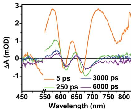
Fig. 8 FSTA spectra of a film of **2** that has been solvent vapor annealed for 10 minutes in  $\text{CH}_2\text{Cl}_2$  showing positive absorptions at 580 and 650 nm resulting from  $^3\text{DPP}$  formation.
