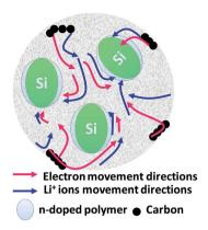
$\label{eq:Fig.6} \textbf{Fig. 6} \quad \text{Silicon nanoparticles with } \ n\text{-doped polymer for volume change} \\ \text{buffering in nano-Si particles}.$
