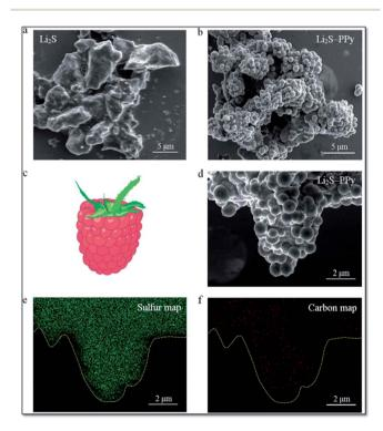
Fig. 11 SEM images of (a) pristine Li<sub>2</sub>S particles and (b) as-synthesized Li<sub>2</sub>S-PPy composite structures. (c) Schematic of a raspberry and (d) SEM image of a representative Li<sub>2</sub>S-PPy raspberry-like composite together with the corresponding elemental maps for (e) sulfur and (f) carbon (reprinted with permission from ref. 246, copyright 2014, Royal Society and Chemical Journal).
