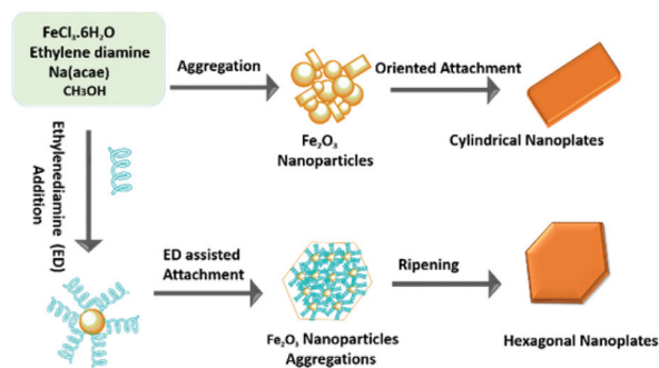
Scheme 1 Schematic illustration of the formation mechanism of hexagonal and cylindrical hematite nanoplates.
