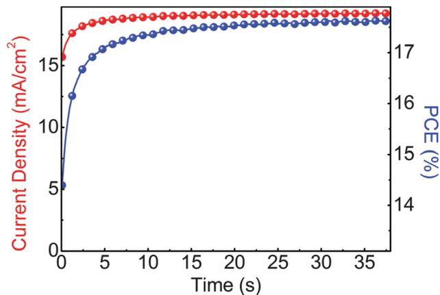
Fig. 3 Stabilized current density and power output measured close to the maximum power point ( $\sim 0.92$  V) for a photovoltaic device of glass/FTO/TiO<sub>x</sub>/60-PCBM/CH<sub>3</sub>NH<sub>3</sub>PbI<sub>3</sub>/spiro-MeOTAD/Au.
