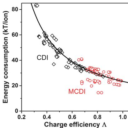
Fig. 5 Data for energy consumption per ion removed, vs. charge efficiency, based on data reported in Zhao *et al.*<sup>26</sup> for CDI and MCDI, for salt inflow concentrations from 5–200 mM. Energy recovery is not included. Divide energy in kT/ion by 200 to convert to MJ mol<sup>-1</sup> salt.
