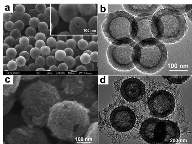
Fig. 5 (a) FESEM and (b) TEM images of HCS-PANI. (c) FESEM and (d) TEM images of GHCS- $\text{MnO}_2$ . Reproduced with permission from ref. 37 and 38. Copyright: 2010 American Chemical Society and 2012 The Royal Society of Chemistry.
