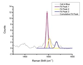
Fig. 4 Representative example of peak fitting for a multiplex spectrum generated from *k*-means cluster analysis (cell 4 blue cluster). Peaks were fitted using a GaussAmp function with constrained parameters resulting in the 3 individual peak fits, Fit 1, 2 and 3 and the overall resultant Cumulative Fit Peak shown overlaid on the original spectrum (black line).
