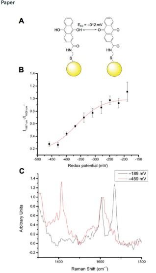
Fig. 2 AQ-NP nanosensor. (A): Equilibrium between oxidised and reduced AQ attached to a gold NP (yellow sphere, not to scale). (B): Calibration curve for AQ-NP nanosensors ( $R^2 = 0.96855$ ). (C): Representative spectra of fully oxidised (-189 mV) and fully reduced (-459 mV) AQ-NPs.
