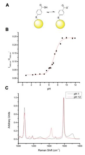
Fig. 1 MBA-NP nanosensor. (A): Equilibrium between protonated and deprotonated MBA attached to a gold NP (yellow sphere, not to scale). (B): Calibration curve for MBA-NP nanosensors ( $R^2 = 0.98687$ ). (C): Representative spectra of fully protonated (pH 1) and fully deprotonated (pH 12) MBA-NPs.
