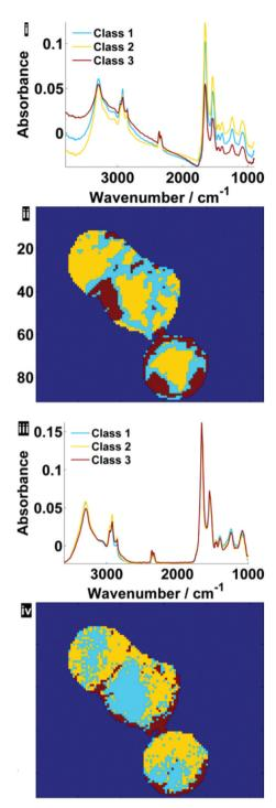
Fig. 7 Pseudo-colour *k*-means cluster maps and mean spectra for 3 classes, displaying different general regions before (i, ii) and after RMieS-EMSC correction (iii, iv).
