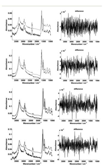
Fig. 5 Typical single pixel spectra illustrating the PCA-based noise reduction algorithm using 50 retained PCs. The high-magnification image representative spectra A-D are shown before and after noise reduction respectively (left). The differences between the raw and corrected spectrum in each case are also displayed (right).
