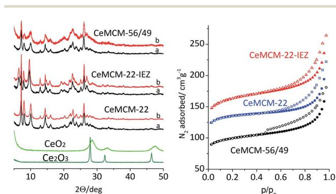
Fig. 1 XRD for  $\text{CeO}_2$ ,  $\text{Ce}_2\text{O}_3$  and Ce-MCM-22, Ce-MCM-22-IEZ, and Ce-MCM-56/49 zeolites, (a) calcined and cerium-exchanged, (b) cerium-exchanged and vacuum activated samples;  $\text{N}_2$  isotherms for calcined samples.
