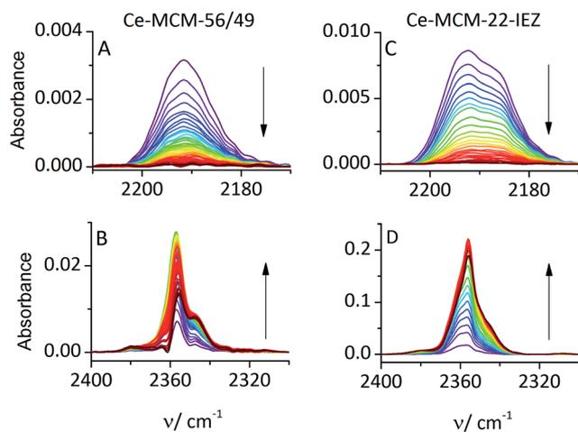
Fig. 3 IR spectra recorded every 15 min in the CO (A and C) and CO<sub>2</sub> region (B and D) for Ce-MCM-56/49 (A and B) and Ce-MCM-22-IEZ (C and D). (Note differences in intensities between upper and lower plots.)
