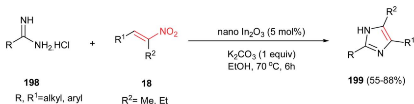
Scheme 67 Synthesis of imidazoles via tandem cyclization between amidine and nitroolefins.
