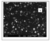
Fig. 1 Particle size and morphology of PEDOT-PSS solution as obtained from (a) TEM & (b) SEM.
