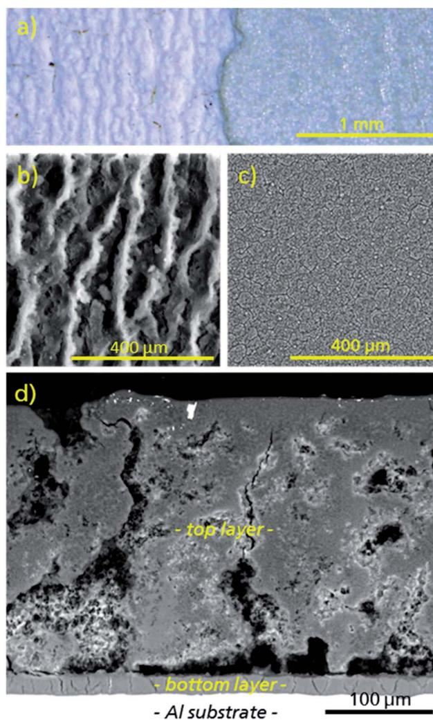
Fig. 7 (a) Representative optical microscope image of the  $\mu\text{p-AF@Al}$  coating in top-down view, with the top layer being removed in the right part of the image in order to expose the bottom layer. The different structures can be seen in (b) (SEM image of the top-down view of the top layer) and (c) (SEM image of the top-down view of the bottom layer), and in the polished cross-section of the whole coating (d).
