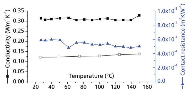
Fig. 10 Thermal conductivity of  $\mu\text{p-AF}$ . Measurements were conducted on bulk  $\mu\text{p-AF}$  (pellet,  $\varnothing = 12.68 \text{ mm}$ ,  $h = 1.71 \text{ mm}$ , forming pressure =  $13 \text{ kN}$ ;  $\rho = 0.714 \text{ g cm}^{-3}$ , empty symbols) and a  $\mu\text{p-AF@Al}$  coated sheet with protective layer (filled symbols). For the  $c_p$  values, the curve determined for bulk  $\mu\text{p-AF}$  was used in both cases (see Fig. S3 in ESI†).
