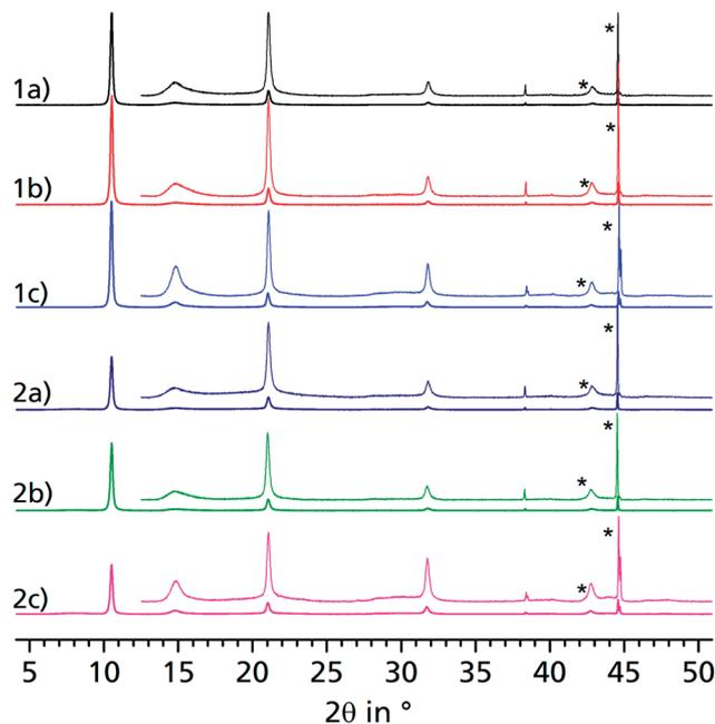
Fig. 8 XRD of two representative  $\mu\text{p-AF@Al}$  sheets 1 and 2, each before cycling (a), after 1500 (b) and 4500 (c) ad-/desorption cycles with water vapour. Sheet 2 has been covered with the silicon resin. Insets are multiplied by the factor of 6 for better visualization. Peaks marked with an asterisk ( $\star$ ) are caused by the Al substrate.
