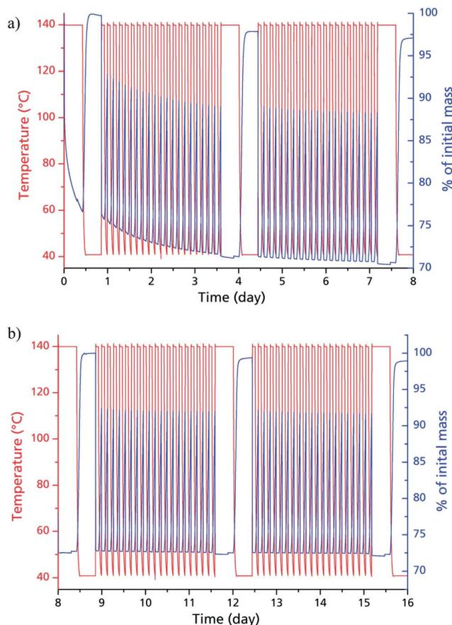
Fig. 5 Thermogravimetric adsorption/desorption cycling experiments for 40 cycles (a), and another 40 cycles (b) of bulk  $\mu\text{p-AF}$ . Long segments at the beginning, in the middle and at the end of each experiment were conducted to determine the equilibrium loading of the sample.
