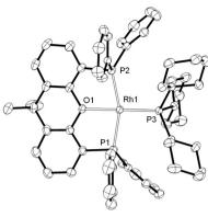
Fig. 4 Solid state structure of the cationic portion of 8. [BAr<sup>F</sup><sub>4</sub>] anion and H atoms are omitted for clarity. Displacement ellipsoids are drawn at the 50% probability level. Selected bond lengths (Å) and angles (°): Rh1-P1,2.2854(7); Rh1-P2,2.2923(7); P3-Rh1, 2.2611(7); Rh1-O1, 2.2395(19); P2-Rh1-P1,159.70(3); P3-Rh1-O1, 170.44(6).
