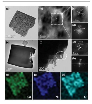
**Fig. 4** (a–d) TEM, HRTEM images and SAED pattern of NiCo $_2$ O $_4$  nanosheets obtained from a hydrothermal reaction time of 3 h; (e–h) TEM, HRTEM images and SAED pattern of NiCo $_2$ O $_4$  hierarchical cubic microstructures consisting of NiCo $_2$ O $_4$  nanosheets obtained from a hydrothermal reaction time of 6 h; and (i–k) The corresponding EDX elemental mapping images of NiCo $_2$ O $_4$  nanosheets obtained from a hydrothermal reaction time of 3 h.
