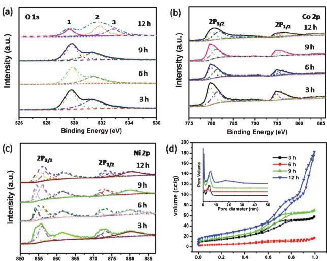
Fig. 6 (a–c) XPS spectra of NiCo<sub>2</sub>O<sub>4</sub> samples at 180  $^{\circ}$ C from different hydrothermal reaction times; (d) N<sub>2</sub> adsorption/desorption isotherms of NiCo<sub>2</sub>O<sub>4</sub> samples with corresponding pore-size distribution (inset).
