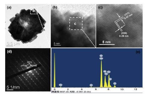
Fig. 5 (a-e) TEM, HRTEM images, SAED pattern and the EDS spectrum of NiCo<sub>2</sub>O<sub>4</sub> hierarchical flower-like super-structures consisting of porous NiCo<sub>2</sub>O<sub>4</sub> nanosheets.
