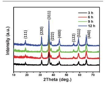
Fig. 2 XRD patterns of  $\rm NiCo_2O_4$  samples at 180  $^{\circ} \rm C$  from different hydrothermal reaction times.
