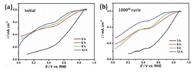
Fig. 7 (a) Linear potential sweep curves for the ORR on NiCo<sub>2</sub>O<sub>4</sub> samples; (b) ORR curves after 1000 cycles on NiCo<sub>2</sub>O<sub>4</sub> samples.
