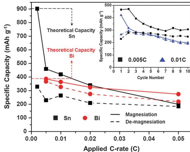
Fig. 2 Magnesianation/de-magnesianation capacities for Sn/Mg (■ black) and Bi/Mg (● red) half-cells at various C-rates. All half-cells were tested using an organohaloaluminate electrolyte. Inset – 10 cycles of a Sn/Mg half-cell at 0.005 C (■ black) and 0.01 C (▲ blue) rates in the same electrolyte.
