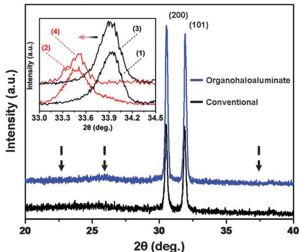
**Fig. 4** XRD spectra of de-magnesiated  $\text{Mg}_2\text{Sn}$  from organohaloaluminate (blue) and conventional (black) electrolytes ( $\text{Mg}_2\text{Sn}$  peak positions marked with arrows). Inset – XRD spectra showing a peak shift due to magnesiation (red) of  $\text{Mo}_6\text{S}_8$  (black) in organohaloaluminate (peak shift 1 → 2) and conventional (peak shift 3 → 4) electrolytes.
