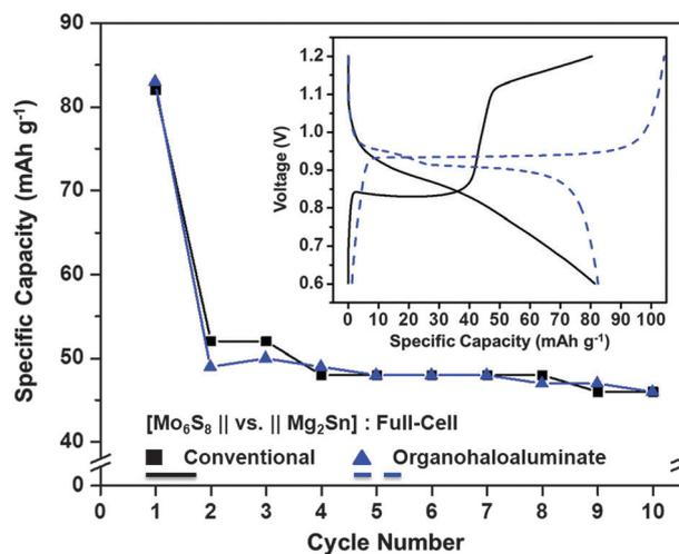
Fig. 3 The first 10 cycles for a  $[\text{Mo}_6\text{S}_8\text{-conventional electrolyte-Mg}_2\text{Sn}]$  full-cell (■ black) and a  $[\text{Mo}_6\text{S}_8\text{-organohaloaluminate electrolyte-Mg}_2\text{Sn}]$  full-cell (▲ blue); inset – 1st cycle voltage profiles for each full-cell.
