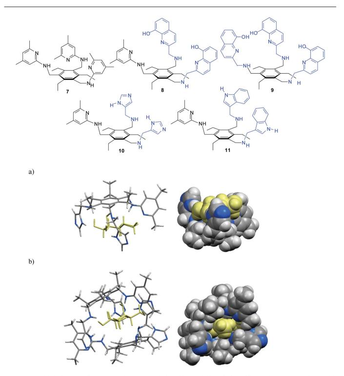
Fig. 2 Energy-minimized structure of the 1:1 (a) and 2:1 complex (b) formed between imidazole/aminopyridine-based receptor 10 and  $\beta$ -galactoside 5b (different representations). MacroModel V.8.5, OPLS-AA force field, MCMM, 50 000 steps. Color code: receptor C, grey; receptor N, blue; sugar molecule, yellow.6g
