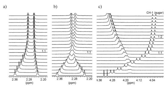
Fig. 5 (a,b) Partial <sup>1</sup>H NMR spectra (400 MHz; CDCl<sub>3</sub>) of receptor 18 before (bottom) and after the addition of  $\beta$ -glucoside 2a (a) and  $\beta$ -galactoside 5a (b); [18] = 0.97 mM, equiv. of 2a or 5a: 0.00–4.80. Shown are pyridine CH<sub>3</sub> resonances of 18. (c) Partial <sup>1</sup>H NMR spectra of sugar 2a before (bottom) and after the addition of receptor 18 (inverse titration); [2a] = 0.78 mM, equiv. of 18: 0.00-4.99.15
