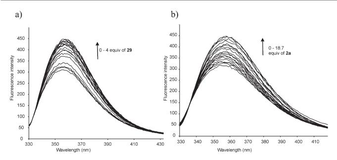
Fig. 7 Fluorescence titration of receptor 26 with α-maltoside 29 (a) and β-glucopyranoside 2a (b) in CHCl<sub>3</sub>; [26] =  $8.51 \times 10^{-5}$  and  $9.57 \times 10^{-5}$  M; Equiv. of 29 = 0.00–4.03; Equiv. of 2a = 0.00–18.69. Excitation wavelength 324 nm. Fluorescence intensity increased with increasing sugar concentration.<sup>24</sup>
