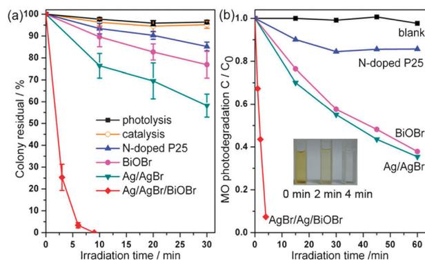
**Fig. 3** Photocatalytic (a) inactivation of *E. coli* and (b) degradation of MO under visible light irradiation ( $\lambda \geq 400 \text{ nm}$ ). The insert demonstrates the color changes of MO over Ag/AgBr/BiOBr hybrid.
