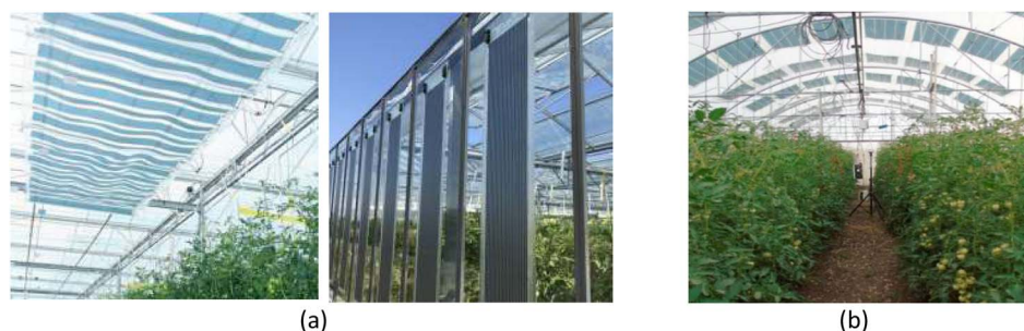
Fig. 6 Flexible OPV modules demonstrated in greenhouses (a) ASCA® modules deployed in an industrial greenhouse, France, reproduced from ref. 77 with permission from ASCA, copyright 2021; (b) testing of OPV modules installed on a polytunnel roof, reproduced from ref. 78 with permission from Elsevier, copyright 2022.
