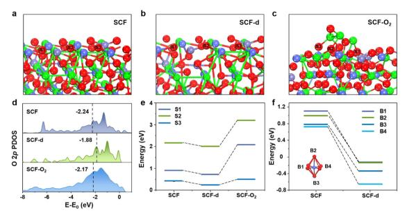
Fig. 3 DFT calculation results. (a)–(c) Models used for the calculation of the O 2p band center and  $E_{vfs}$  for the (222) facet of (a) SCF, (b) SCF-d and (c) SCF-O<sub>2</sub>. (d) PDOS diagrams of the O 2p band and the calculated band center relative to the Fermi level, (e)  $E_{VfS}$  of different sites in SCF, SCF-d and  $SCF-O_2$  and (f)  $E_{vfb}$  of different sites in SCF and SCF-d. Color code: O (red ball), Sr (green ball), Co (dark blue ball), and Fe (light blue ball)
