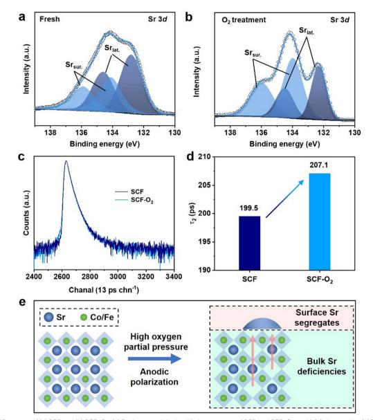
Fig. 1 Sr 3d XPS spectra of (a) SCF and (b) SCF-O<sub>2</sub>. (c) Positron annihilation lifetime spectra of SCF and SCF-O<sub>2</sub> and (d) fitting results. (e) The schematic of Sr segregation to generate surface Sr segregates and bulk Sr deficiencies.
