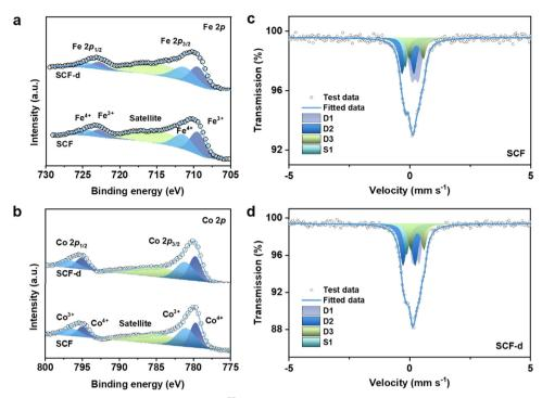
Fig. 2 XPS spectra of (a) Fe 2p and (b) Co 2p of SCF and SCF-d. <sup>57</sup>Fe Mossbaüer spectra of (c) SCF and (d) SCF-d samples.
