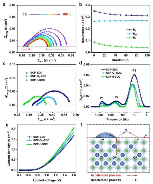
Fig. 5 The electrochemical performances of SOECs with different anodes at 800 °C. (a) and (b) EIS spectra of an SCF-SDC symmetrical cell immersed in an O<sub>2</sub> atmosphere at 800 °C for 100 hours. (c) EIS spectra of single cells with different anodes at 1.2 V and (d) the DRT fitting results. (e) Current densityvoltage curves (J-V) at 800 °C. (f) A schematic illustration of Sr segregation.
