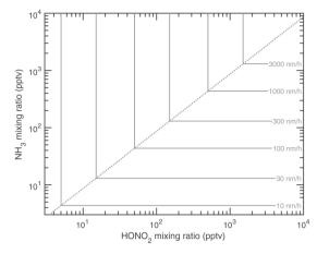
Fig. 9 Maximum growth rates of 10 nm particles at 263 K for ammonium nitrate formation. Growth rates are shown as contour labels. The maximum depends sharply on the limiting vapor, with ammonia limitation causing horizontal contours at relatively high nitric acid and nitric acid limitation causing vertical contours at relatively high ammonia. The spine is offset from 1:1 based on the relative vapor speeds and depends on particle size
