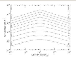
Fig. 14 Growth rate at 10 nm vs. the collision ratio for different excess saturation ratios (on contour labels) at 263 K (with no Kelvin term, i.e.  $d_{\rm K10}=1$ ). At modest  $S_{\rm AB}^{\rm xs} \lesssim 10$ , the depression in  $\gamma$  for  $r_{\rm AB}^{\rm xs} \simeq 1$  rounds the growth rate curve in the center, whereas for greater saturation it remains sharp.
