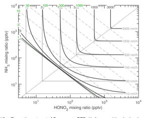
Fig. 15 Growth rate at 10 nm at 278 K (top, with dashed purple saturation ratio diagonal lines) and 263 K (bottom, with dashed green saturation ratio diagonal lines). These are the two temperatures shown for CLOUD data in Fig. 1. As with the "natural" growth coordinates, near the 1:1 equi-collision spine the growth rate is rounded compared to the sharp limiting values, with contours converging toward no growth at the S=1 saturation diagonal line.
