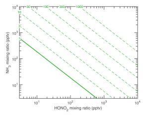
Fig. 10 Saturation ratio over a pure ammonium nitrate crystalline surface at 263 K vs. nitric acid and ammonia mixing ratios. The solid green diagonal shows S=1. Regions to the lower left are undersaturated and particles will evaporate; those to the upper right, with saturation ratios indicated on the dashed contours, are super saturated and particles will grow. The saturation threshold moves toward the lower left as temperature falls and towards the upper right as it increases.
