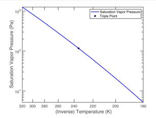
Fig. 4 Saturation vapor pressure of nitric acid over a pure liquid.
