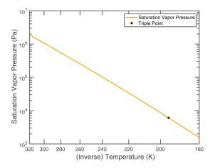
Fig. 2 Saturation vapor pressure of ammonia over a pure liquid.
