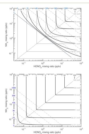
Fig. 16 Growth rate of 10 nm particles at 243 K (top) and 223 K (bottom). Note the axes shift by a factor of 100 compared to the warmer Fig. 15. At 223 K (i.e. in the upper troposphere), the only sign of reversible (semi-volatile) condensation by the limiting reagent is curvature near the equi-collision spine with both vapors below a 1 pptv mixing ratio and almost imperceptible growth of 0.1 nm  $h^{-1}$ .
