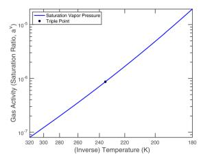
Fig. 5 Saturation ratio (gas-phase activity) of 1 ppbv of nitric acid over a pure liquid.
