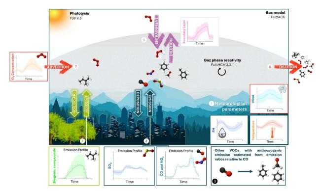
Fig. 1 Description of the scenario implemented in the box model to reproduce the urban environment: emissions, deposition, boundary layer height, advection/dilution, and meteorological parameters (T, P, RH, and wind speed).
