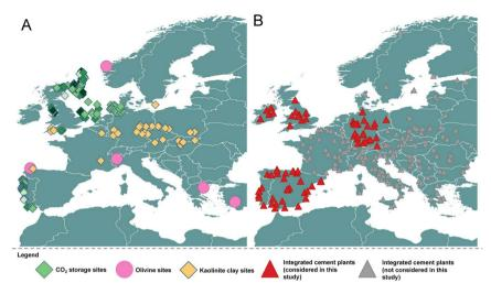
Fig. 2 Available locations for production of olivine-bearing rocks<sup>23</sup> and kaolinite clays<sup>24–26</sup> and for offshore  $CO_2$  storage<sup>27,28</sup> of relevance for the here analysed regions (*i.e.*, Ireland, United Kingdom, Germany, Portugal and Spain) (A). Integrated cement plant locations in Europe<sup>22</sup> (B). Regions analysed in this study are marked in red.
