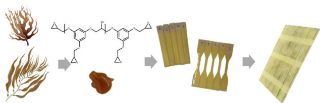
Scheme 1 Chemical formula of PHTE and the so-formed resin and glass fibre reinforced composite images.
