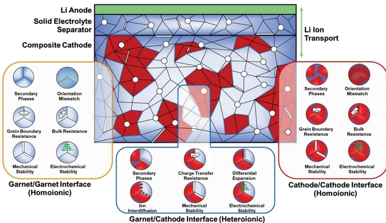
Fig. 8 The various structural, chemical, electrochemical and mechanical properties at the garnet–cathode interface that evolve during operation illustrated in the composite cathode design.<sup>121</sup> Copyright 2022, John Wiley and Sons.
