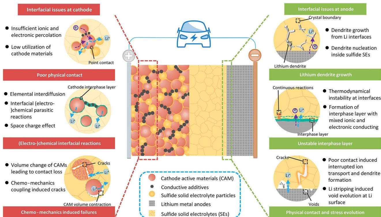
Fig. 7 Illustration of various interfacial challenges at cathode and anode interfaces with solid electrolytes in ASSBs.<sup>120</sup> Copyright 2022 John Wiley and Sons.
