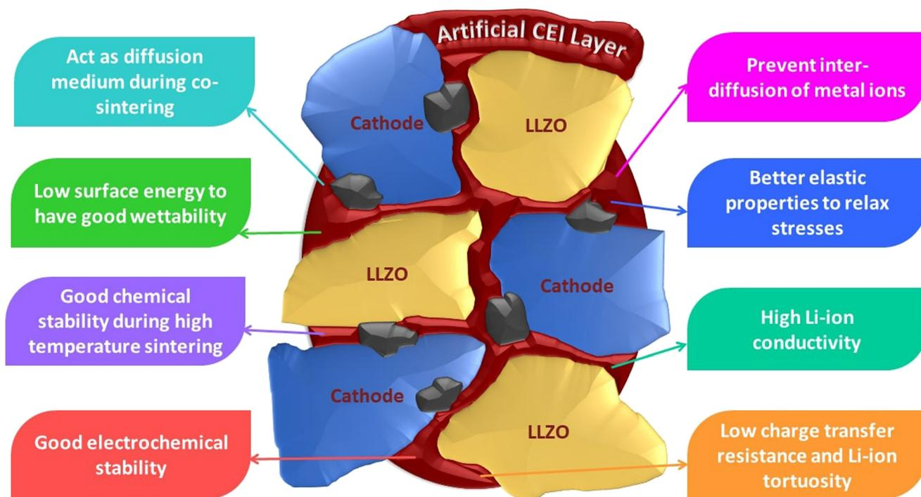
Fig. 12 Properties of an artificial CEI layer.
