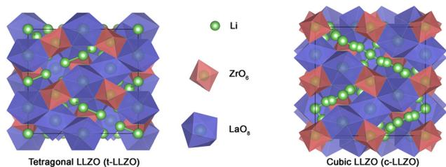
Fig. 1 The crystallographic structure of tetragonal and cubic LLZO projected along the normal to the (100) plane.
