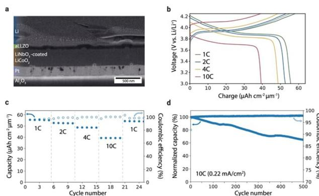
Fig. 13 (a) Cross-section SEM image of the battery stack. (b) Charge–discharge curves at different C rates ( $1\text{C} = 22 \mu\text{A cm}^{-2}$ ). (c) Discharge capacity and coulombic efficiency of the battery at different C rates. (d) Long-term cycling of the battery over 500 cycles at  $10\text{C}$  ( $0.22 \text{ mA cm}^{-2}$ ).<sup>160</sup> Copyright 2021 Springer Nature Limited.
