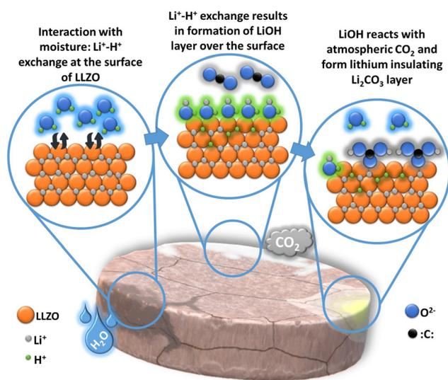
Fig. 5 Surface reactions on an LLZO pellet in ambient atmosphere. Initially,  $\text{Li}^+/\text{H}^+$  exchange happens in the presence of moisture, replacing lithium in LLZO with hydrogen. As a result a thin layer of  $\text{LiOH}$  is formed at the surface. This thin layer of  $\text{LiOH}$  interacts with atmospheric  $\text{CO}_2$  to form a thin lithium insulating layer of  $\text{Li}_2\text{CO}_3$ .
