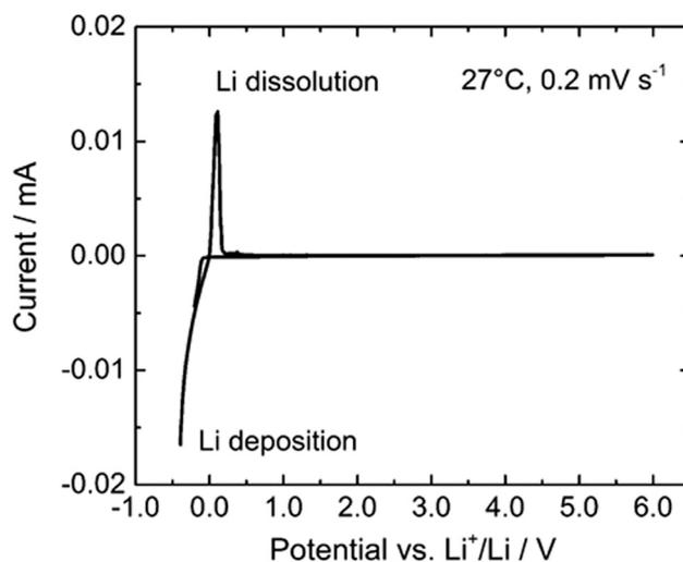
Fig. 6 Cyclic voltammogram of  $\text{Li}_{6.5}\text{La}_{2.8}\text{Ba}_{0.2}\text{Zr}_{1.3}\text{Ta}_{0.7}\text{O}_{12}$  measured at a scanning rate of  $0.2$  mV  $\text{s}^{-1}$  at  $27$  °C.<sup>55</sup> Copyright 2016 Frontiers Media S.A.
