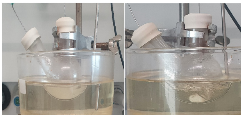
Scheme 1 (Top) The “derivative” switchable solvent method to solubilise cellulose. (Bottom) The dissolution of cellulose in a DMSO/DBU/CO 2 mixture. Photo PMN, 2022.
