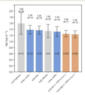
Fig. 2 Annual mean atmospheric Hg<sup>0</sup> concentration at each station type across Switzerland. The blue bars indicate urban sites and the brown bars rural sites, respectively. The rural highway sites and the high altitude site (gray bars) were not assigned to either group. Error bars represent the standard deviation from the mean. The number of measurements is given for each station type
