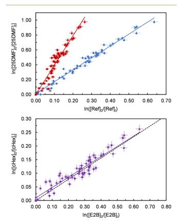
Fig. 1 Relative-rate plots of the 2,5-dimethylfuran +  $O_3$  system using cyclohexene (red) and E2-butene (blue) as references (upper panel) and the crosscheck of both references (lower panel) using the PTR-MS data. The dotted line represents the theoretically expected rate coefficient ratio. Different experimental runs are denoted with different symbols. Error bars represent the  $2\sigma$  statistical uncertainty.
