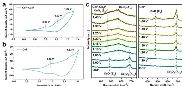
**Fig. 3** (a) CV curve in the potential range of 0.4–1.3 V vs. RHE of CoP–Cu<sub>3</sub>P, with a scan rate of 5 mV s<sup>-1</sup>. (b) CV curve in the potential range of 0.7–1.6 V vs. RHE of CoP, with a scan rate of 5 mV s<sup>-1</sup>. (c) *In situ* Raman spectroscopy conducted on the CoP–Cu<sub>3</sub>P electrode at increasing applied potentials from OCP to 1.4 V (left) and on the CoP electrode at increasing applied potentials from OCP to 1.6 V (right).
