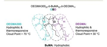
**Fig. 1** Chemical structure of the thermoresponsive polymer OEGMA300 $_{20}$ -b-BuMA $_{22}$ -b-DEGMA $_{11}$  (OBD), with hydrophilic OEGMA300 units shown in cyan, hydrophobic BuMA units in black, and thermoresponsive DEGMA units in purple.
