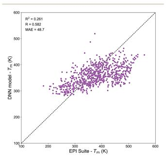
Fig. 9 Correlation plot between the  $T_{\rm m}$  values predicted by the DNN model and by the MPBPWIN module of EPI Suite for SOA compounds from Shiraiwa et al.56
