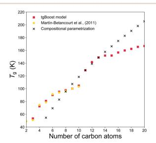
Fig. 3  $T_{\rm g}$  values predicted for the n-alkanes (n=2-20) by the developed tgBoost model (red dots), molecular dynamics simulations (yellow squares),<sup>38</sup> the  $T_{\rm g}$  compositional parametrizations (black crosses).<sup>8</sup>
