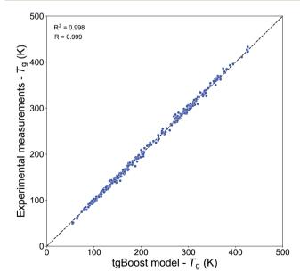
Fig. 2 Correlation plot between the predicted  $T_{\rm g}$  values by the tgBoost model and the experimental  $T_{\rm g}$  values from the  $T_{\rm g}$ -Measured dataset.
