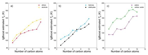
Fig. 6 Estimated  $T_q$  of weakly functionalized isomeric molecules by functional group as a function of the number of carbon atom within the molecule. Isomers are grouped as (a) ethers and alcohols, (b) ketones and aldehydes, and (c) esters and carboxylic acids. The respective functional groups are positioned at the end of the alkyl chain for all species.
