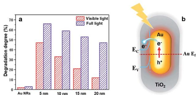
Fig. 5 (a) Photocatalytic degradation of methylene blue by Au NR@TiO<sub>2</sub> core-shell nanostructures with different shell thicknesses under full light and visible light illumination. (b) Mechanistic diagram of Au NR@TiO<sub>2</sub> core-shell nanostructure enhanced photocatalysis under illumination.
