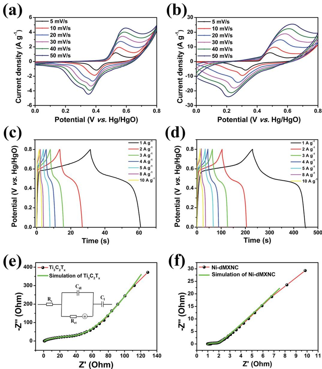
Fig. 5 CV curves of the (a)  $\text{Ti}_3\text{C}_2\text{T}_x$  and (b) Ni-dMXNC electrodes at various scan rates; GCD curves of the (c)  $\text{Ti}_3\text{C}_2\text{T}_x$  and (d) Ni-dMXNC electrodes at various scan rates and current densities. EIS of the (e)  $\text{Ti}_3\text{C}_2\text{T}_x$  and (f) Ni-dMXNC electrodes.
