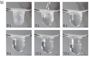
Fig. 10 (a) PCL-BTA/B (1 wt%) has been processed into cup-shaped objects by thermoforming, whereas pristine PCL can only be thermoformed with the aid of a paper support. (b) The PCL-BTA/B cups were filled with boiling water. Defects associated with the connection of the mold to the vacuum pump during thermoforming resulted in water leakage after 12 s but the cups remained globally intact. Scale bars represent 1 cm.
