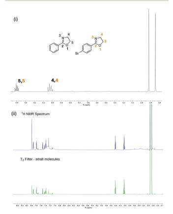
Fig. 4 (i) Partial <sup>1</sup>H NMR spectrum (400 MHz, CDCl<sub>3</sub>) of copolymerisation of 1 and 8, showing overlap of the signals corresponding to monomers. (ii) <sup>1</sup>H NMR spectrum (400 MHz, CDCl<sub>3</sub>) of the same reaction mixture with  $T_2$  filter applied.
