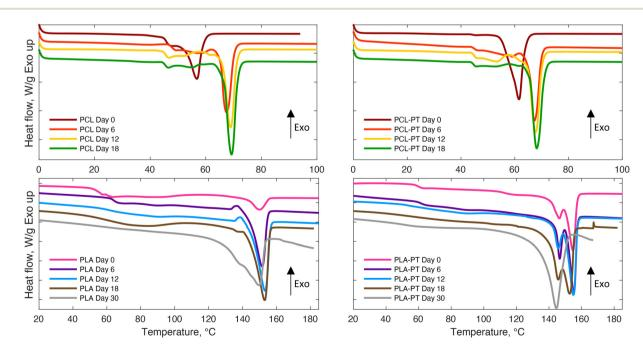
Fig. 4 Differential scanning calorimetry of PCL (top left), PCL pretreated (top right), PLA (bottom left), and PLA pretreated (bottom right) for day 0 and during the early stage of the biodegradation process.
