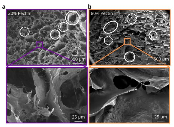
Fig. 5 Effects of adding pectin on morphological properties. SEM images of a CADES BC foam with (a) 20% pectin and (b) 80% pectin at 30x (top row) and 500x (bottom row) magnifications. Solid circles indicate cells in the foams, dashed circles indicate holes in the matrix.
