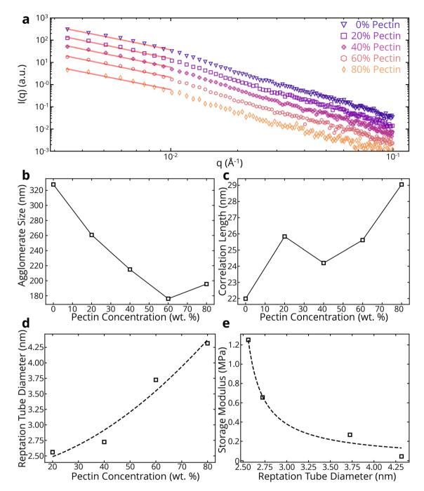
Fig. 4 Effects of adding pectin on network properties via SAXS. (a) SAXS data for CADES BC/pectin composites with a power-law fit in the low-q region. (b) Agglomerate size, (c) correlation length, (d) and reptation tube diameter of CADES BC/pectin composites. (e) Effect of reptation tube diameter on storage modulus of the colloids.
